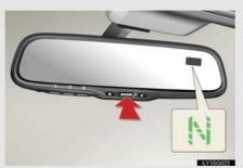
To turn the compass on or off, press "AUTO" for 3 seconds.
