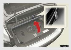
The lever can be hooked on the edge of the trunk.
