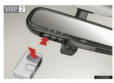
Press and hold one of the buttons on the HomeLink<sup>®</sup> and the button on the transmitter. When the indicator light on the HomeLink<sup>®</sup> changes from a slow to a rapid flash after 20 seconds, you can release both buttons.
