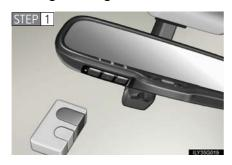
Point the remote control for the device 1 to 3 in. (25 to 75 mm) from the HomeLink  $^{\circledR}$  control but-
