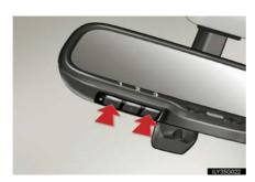
Press and hold the 2 outside buttons for 20 seconds until the indicator light flashes.
