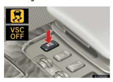
Push and hold the button for more than 3 seconds while the vehicle is stopped to turn off TRAC and VSC.
