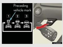
Each pull of the switch changes the vehicle-to-vehicle distance
