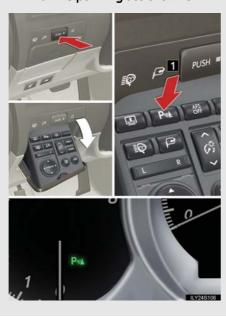
11 Press the switch to turn the system on/off.
