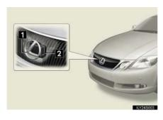
Detects vehicles or other obstacles on or near the road ahead and determines whether a collision is imminent based on the position, speed, and heading of the obstacles.
