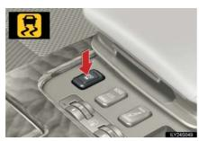
Quickly push and release the button to turn off TRAC.
