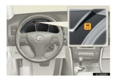
If the vehicle is in danger of slipping, rolling backwards when starting on an incline, or if the rear wheels (2WD models) or all wheels (4WD models) spin, the slip indicator light flashes to indicate that the VSC/TRAC/hill-start assist control systems have been engaged.
