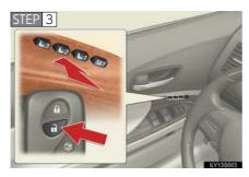
Push the "1", "2" or "3" button on the driver's side and the button on the wireless remote control at the same time for about 1 second until you hear a beep.
