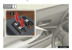
Shift the shift lever to "P" or "N", press and hold the driver's door lock switch (11 or 22) for approximately 5 seconds then release.
