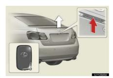
Press the button to unlock the trunk.
