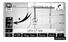
When the vehicle is on the guidance route, the distance and the estimated travel/arrival time to the destination are displayed. When the vehicle is not on the guidance route, the distance and the direction of the destination are displayed.
