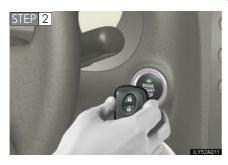
Touch the Lexus emblem side of the electronic key to the engine switch.
