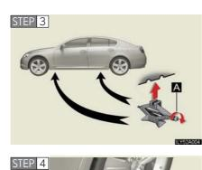
Turn the tire jack portion "A" by hand until the notch of the jack is in contact with the jack point.
