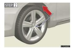
Slightly loosen the wheel nuts (one turn).
