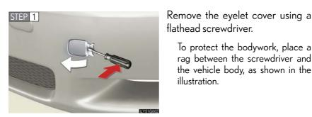
To protect the bodywork, place a rag between the screwdriver and
