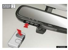
Press and hold down one of the buttons on the HomeLink<sup>®</sup> and the button on the transmitter. When the indicator light on the HomeLink<sup>®</sup> changes from a slow to a rapid flash after 20 seconds, you can release both buttons.
