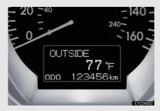
Push the "DISP" button on the steering switch.  $(\rightarrow P. 113)$
