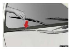
Lower the wipers by pressing on the upper part of the hook section.
