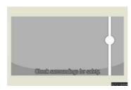
If a bright light (for example, sunlight reflected off the vehicle body) is picked up by the camera, a smear effect\* peculiar to the camera may occur.
