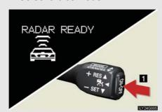
Selecting vehicle-to-vehicle distance control mode
