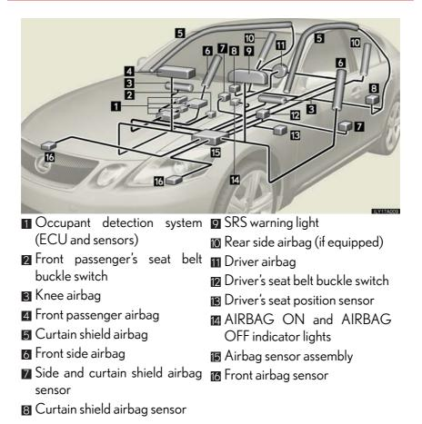
Your vehicle is equipped with ADVANCED AIRBAGS designed based on US motor vehicle safety standards (FMVSS208). The airbag system controls airbag deployment power for the driver and front passenger. The driver airbag system consists of the driver seat's position sensor etc. The front passenger's airbag system consists of the front passenger occupant classification sensor etc.
