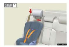
Secure the child restraint using a seat belt or lower anchors, and lock the head restraint in place at the lowest position.
