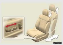
Head restraint height can be adjusted automatically along with the seat position adjustment.  $(\rightarrow P. 25)$
