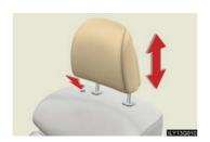
Push and hold the lock release button when lowering or raising the head restraint.
