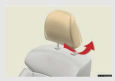
Grip head restraint and twist to tilt forward or backward.
