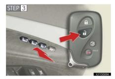
Push the "1", "2" or "3" button on the driver's side and the abutton on the wireless remote control at the same time for about 1 second until you hear a beep.
