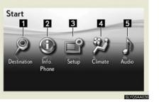
Push the "MENU" button on the Remote Touch to display the "Start" screen.
