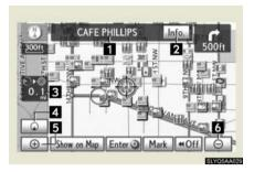
To scroll over the map, place the pointer in a position near the desired destination and then press and hold the "ENTER" button on the Remote Touch.
