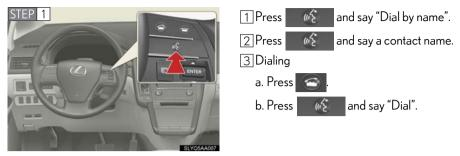
: Pressing this switch turns the voice command system on. Say a command after the beep.
