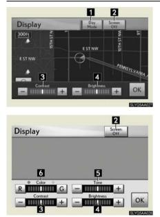
Push the "DISP" button on the Remote Touch to show the "Display" screen.
