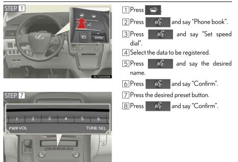
: Pressing this switch turns the voice command system on. Say a command after the beep.
