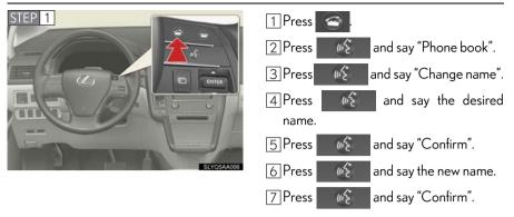
: Pressing this switch turns the voice command system on. Say a command after the beep.
