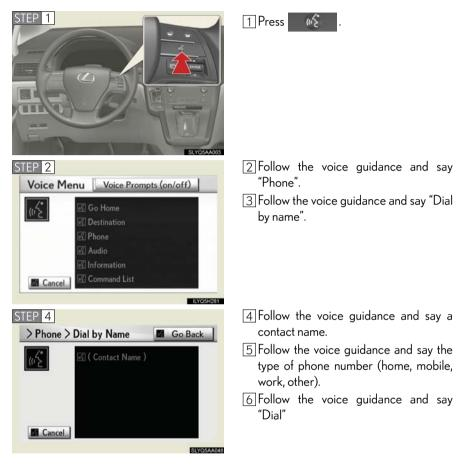
Pressing this switch turns the voice command system on. Say a command after the beep.
