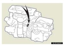
The engine numbers is stamped on the engine block as shown.
