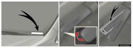
This number is stamped on the top left of the instrument panel and under the front passenger's seat (on some models).
