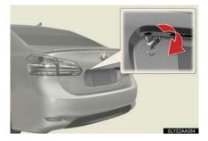
Turn the mechanical key clockwise to open.
