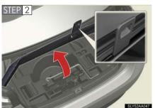
Secure the panel using the hook provided.
