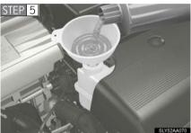
Check that the coolant level of the power control unit is between the "FULL" and "LOW" lines of the reservoir tank.
