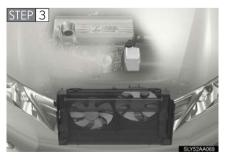
Wait until the hybrid system has fully cooled down. When the system has fully cooled down, check if coolant has leaked from the radiator core.
