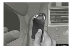
STEP 3 To change "POWER" switch modes: Within 10 seconds of the buzzer sounding, release the brake pedal and press the "POWER" switch. Modes can be changed each time the switch is pressed. (→P. 153)
