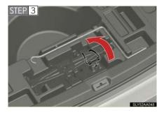
Remove the jack after removing the hook.
