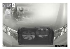
After the hybrid system has cooled down sufficiently, check the engine coolant level and inspect the cooling system for leaks.
