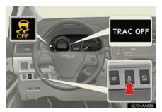
To turn the TRAC and VSC systems off, press and hold the button for more than 3 seconds while the vehicle is stopped.
