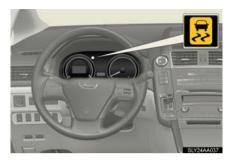
If the vehicle is in danger of slipping or if any of the drive wheels spins, the slip indicator light flashes to indicate that the VSC/TRAC systems are operating.
