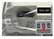
To turn the TRAC system off, quickly press and release the button.
