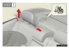
Secure the child restraint system using the seat belt or the LATCH anchors, and remove the head restraint.
