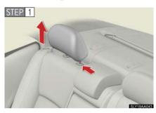
Remove the head restraint.
