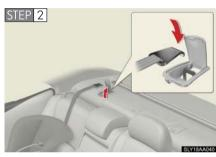
Open the anchor bracket cover, latch the hook onto the anchor bracket and tighten the top tether strap.
