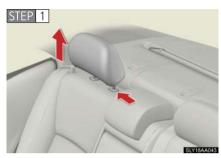
Remove the head restraint.
