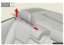
Remove the head restraint.
