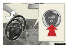
When the "POWFR" switch is turned off, the steering wheel returns to its stowed position by moving up and away to enable easier driver entry and exit.
