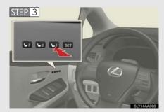
Press button 1, 2 or 3 until the signal beeps to recall the desired position.
