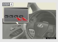
While pressing and holding the "SET" button, or within 3 seconds of pressing the "SET" button, press button 1, 2 or 3 until the signal beeps.
