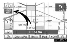
When your vehicle is receiving signals from the satellites, the "GPS" mark appears at the top left of the screen.
