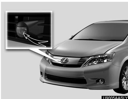
The wide view front monitor system camera is located on the front grille as shown in the illustration.
