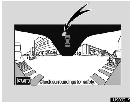
If the wide view front monitor is switched to from the intuitive parking assist, the icon display area will flash to inform the driver that the currently displayed area is the front. The icon display area will continue to flash until the screen is turned off.
