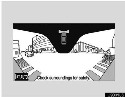
The image from the front camera is displayed. Use this monitor to help check the area in front of the vehicle for safety, for example in intersections with poor visibility.
