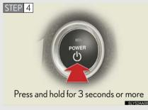
Stop the hybrid system by pressing and holding the "POWER" switch for 3 consecutive seconds or more.
