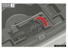
Remove the jack after removing the hook.
