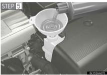
Add power control unit coolant if necessary.
