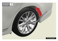
Slightly loosen the wheel nuts (one turn).
