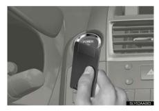
STEP 3 To change "POWER" switch modes: Within 10 seconds of the buzzer sounding, release the brake pedal and press the "POWER" switch. Modes can be changed each time the switch is pressed. (→P. 148)
