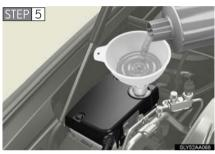
Add engine coolant if necessary.
