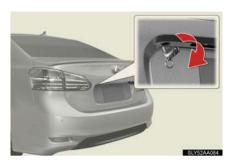
Turn the mechanical key clockwise to open.
