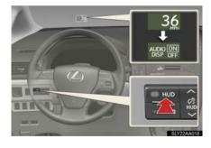
With the touch tracer display ON/ OFF selection mode displayed, press and hold HUD (Head-up Display) main switch for more than 2 seconds again to enter audio display ON/OFF selection mode. ON or OFF can be selected by pressing HUD (Head-up Display) main switch.
