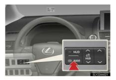
Pressing the switch turns the turnby-turn navigation on/off, when the head-up display is on.
