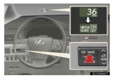
Pressing and holding the HUD (Head-up Display) main switch for more than 2 seconds changes the display to touch tracer display ON/OFF mode. Press the HUD (Head-up Display) main switch to select ON or OFF.
