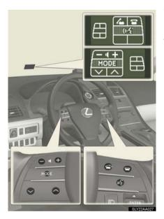
The display will change in response to steering switch operation.
