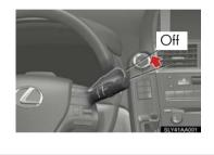
Set the wiper switch to the off position. If the wiper switch is in "AUTO", the wipers may operate and the wiper blades may be
