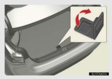
Pull the lever upward to lift up the luggage mat.
