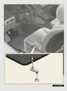
Secure the floor mat using the hooks provided.
