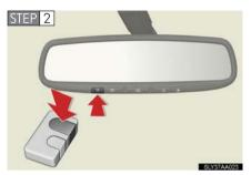
Press and hold one of the HomeLink<sup>®</sup> buttons and the transmitter button. When the HomeLink<sup>®</sup> indicator light changes from a slow to a rapid flash after 20 seconds, release both buttons.
