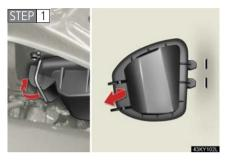
Release the lock and remove the cover.
