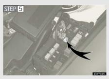
Remove the fuse with the pullout tool.
