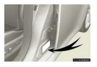
For the GAWR, see the Certification Label. For the maximum load of the tire, see the load limit at maximum cold tire inflation pressure mentioned on the sidewall of the tire. ( $\rightarrow$ P. 530)
