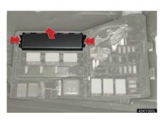
Lift the lid off while pushing the tabs on either side.
