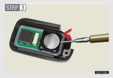
Remove the depleted battery.
