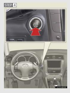
Press the "ENGINE START STOP" switch.
