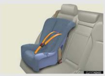
Seat belts equipped with a child restraint locking mechanism (ALR/ELR belts except driver's seat belt) (→P. 66)
