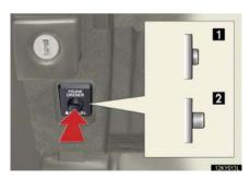
Turn the trunk opener main switch in the glove box off to disable the trunk opener.
