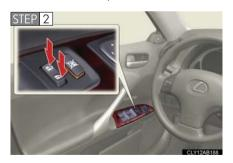
Shift the shift lever to P or N, press and hold the driver's door lock switch ( or or of ) for about 5 seconds then release.
