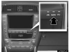
1. Push the air intake control button until the "Adjust Exhaust Gas Sensor" screen appears while the vehicle is stopped.
