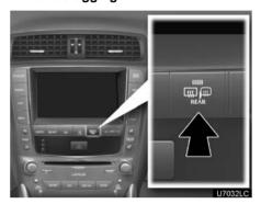
To turn the electric rear window and outside rear view mirror defogger on, push the button above.
