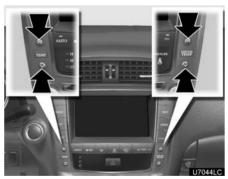
Push the " $\wedge$ " button on "TEMP" to increase the temperature and " $\vee$ " to decrease the temperature.
