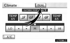
"DUAL" button is used to set the temperatures independently for the driver's seat and front passenger seat.
