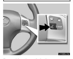
By pushing the switch above, you can operate the voice command system.
