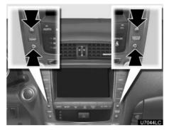
To adjust the temperature setting, push the " $\wedge$ " button on "TEMP" to increase the temperature and push the " $\vee$ " button to decrease the temperature.
