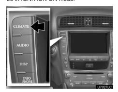
Push the "CLIMATE" button to display the air conditioning control screen.
