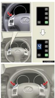
1 Pull the "-" shift paddle switch toward you. The indicator in the meter cluster will display the selected shift range.
