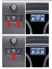
1 To cycle through the functions, press either the left or right selector switch.
