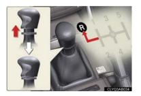
To operate the shift lever, the clutch pedal must be fully depressed.
