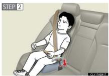
Sit the child in the booster seat. Fit the seat belt to the booster seat according to the manufacturer's instructions and insert the plate into the buckle. Make sure that the belt is not twisted.
