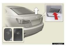
Press the button to unlock the trunk.
