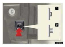
Turn the trunk opener main switch in the glove box off to disable the trunk opener.
