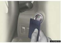
Touch the Lexus emblem side of electronic the kev to the "ENGINE START STOP" switch.
