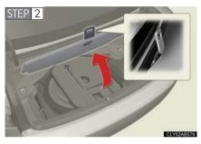
Secure the panel using the hook provided.
