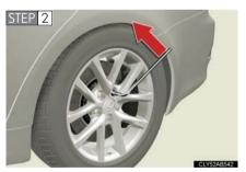
Slightly loosen the wheel nuts (one turn).
