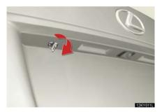
Turn the mechanical key clockwise to open.
