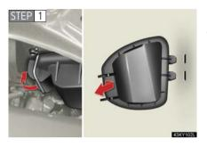
Release the lock and remove the cover.
