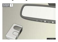
Point the remote control transmitter for the device 1 to 3 in. (25 to 75 mm) from the HomeLink<sup>®</sup> buttons.
