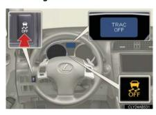
Push and hold the switch for more than 3 seconds or more while the vehicle is stopped to turn off TRAC and VSC.
