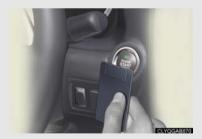
If the electronic key battery becomes depleted, replace it with a new battery. For instructions on replacing the battery, refer to the Owner's Manual. If you need further assistance, contact your Lexus dealer.
