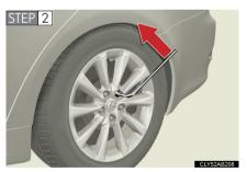
Slightly loosen the wheel nuts (one turn).
