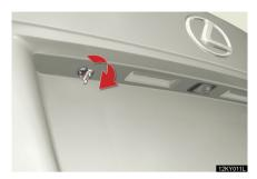
Turn the mechanical key clockwise to open.
