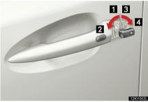
Remove the cover on the driver's door handle using the mechanical key ( $\rightarrow$ P. 25) in order to perform the following operations.
