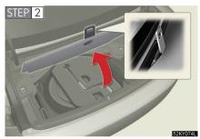
Secure the panel using the hook provided.
