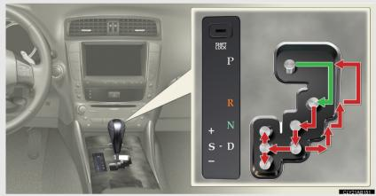
While the "ENGINE START STOP" switch is in IGNITION ON mode, depress the brake pedal and move the shift lever.
