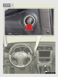
Press the "ENGINE START STOP" switch.
