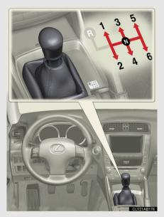
Fully depress the clutch pedal before operating the shift lever, and then release it slowly.
