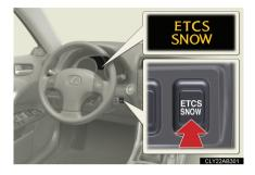
The snow mode is used for accelerating and driving on slippery road surfaces, such as on snow.
