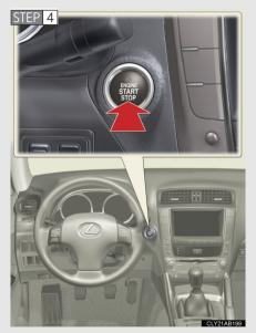
Press the "ENGINE START STOP" switch.
