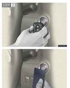
Touch the Lexus emblem side of the electronic key to the "ENGINE START STOP" switch.
