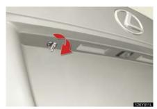
Turn the mechanical key clockwise to open.
