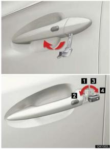
Remove the cover on the driver's door handle using the mechanical key (→P. 21) in order to perform the following operations.
