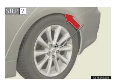
Slightly loosen the wheel nuts (one turn).
