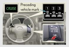
Each push of the switch changes the vehicle-to-vehicle distance
