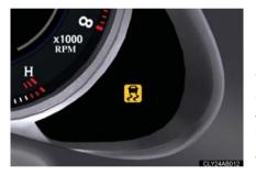
If the vehicle is in danger of slipping, rolling backwards when starting on an incline, or if the rear wheels (2WD) or 4 wheels (AWD) spin, the slip indicator light flashes to indicate that the VSC/ TRAC/hill-start assist control systems have been engaged.
