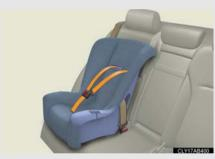
Seat belts equipped with a child restraint locking mechanism (ALR/ELR belts except driver's seat belt) (→P. 56)
