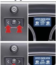
1 To cycle through the functions, press either the left or right selector switch.
