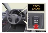
An indicator comes on when in snow mode. Press again to return to normal mode.
