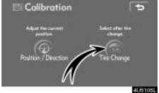
To perform a distance calibration procedure, touch "Tire Change" on the "Calibration" screen.
