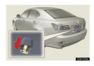
The trunk lid can be opened by pulling down on the glow-in-the-dark lever located on the inside of trunk lid.
