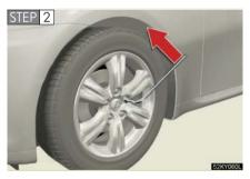
Slightly loosen the wheel nuts (one turn).
