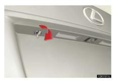
Turn the mechanical key clockwise to open.
