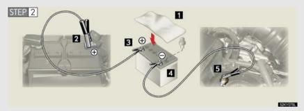
Connecting the jumper cables.
