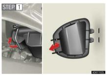
Release the lock and remove the cover.
