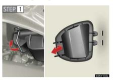
Release the lock and remove the cover.
