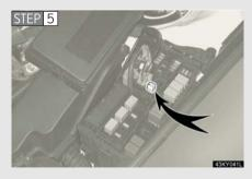
Remove the fuse with the pullout tool.
