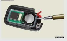
Remove the depleted battery.
