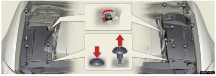
n Installing the clips
