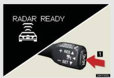
Selecting vehicle-to-vehicle distance control mode
