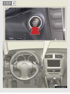
Press the "ENGINE START STOP" switch.
