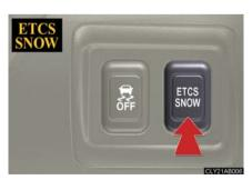
The snow mode is used for accelerating and driving on slippery road surfaces, such as on snow.
