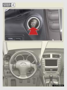
Press the "ENGINE START STOP" switch.
