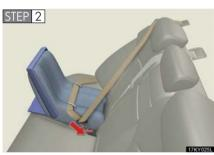
Run the seat belt through the child seat and insert the plate into the buckle. Make sure that the belt is not twisted.
