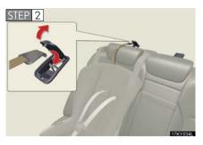
Open the anchor bracket cover, latch the hook onto the anchor bracket and tighten the top strap.
