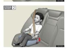
Sit the child in the booster seat. Fit the seat belt to the booster seat according to the manufacturer's instructions and insert the plate into the buckle. Make sure that the belt is not twisted.
